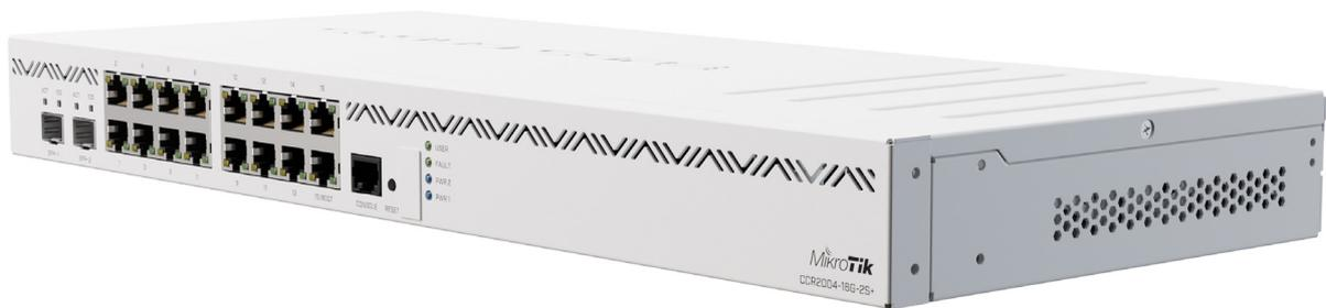
The new router has 18 wired ports, including 16x Gigabit Ethernet ports and two 10G SFP+ cages. It also has a RJ-45 console port on the front panel.
